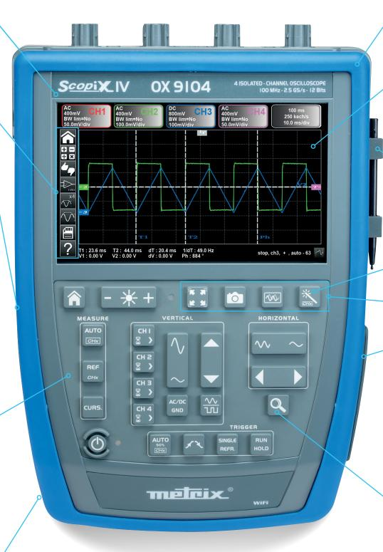
To allow you to work in peace, there is no longer a fan: the heat is dissipated by conduction through the internal components of the SCOPIX IV models.
