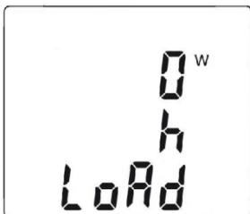
8. To access the screens concerning the energies generated by the load and therefore received by the source ("Supply side"), press the
