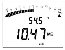
The A symbol indicates that the instrument is generating a hazardous voltage (> 70 V).
