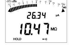
Then long-press the **MEM** key to store the measurement. The measurement is recorded in the first memory slot
