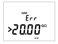
With the CA 6532, if this occurs during a DAR or PI measurement, the instrument interrupts the measurement and displays the screen shown opposite.
