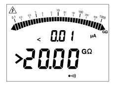
If, during an insulation measurement, the value to be measured exceeds the measurement range (which depends on the instrument and the test voltage), the instrument so reports.
