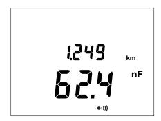
The instrument displays the capacitance and the corresponding line length, computed from the programmed capacitance per unit length.
